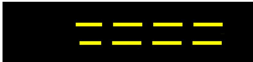
4. **Runway Holding Position Markings** – Yellow. Identified by two solid and two dashed yellow lines located on taxiways that access a runway. The dashed lines indicate the runway side of the marking. These lines indicate the edge of the protected area around a runway and are accompanied by runway hold position signs. Runway Holding Position Markings apply to: aircraft, vehicles, and personnel.
